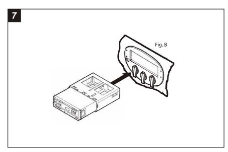
**DIN HEAD UNITS:** Slide the DIN cage into the Integrated Mounting Kit and secure by bending the metal locking tabs down. Slide the aftermarket head unit into the cage until secure. (see Fig. B)
